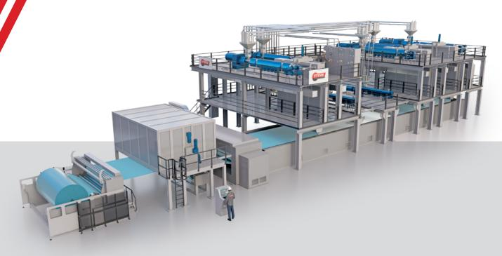
The polymer in the form of granules or flakes is extruded through our equipment to form continuous filaments which are conditioned, drawn and deposited over a suitable moving surface (forming belt), creating a web. Suitable downstream equipment is provided to make the finishing/consolidation in accordance to the final application.
